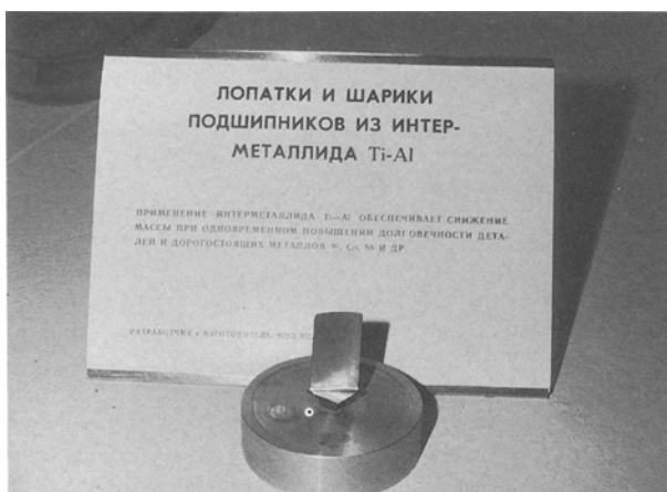
Figure 21 Turbine blade produced from TiAl using a powder metallurgy and hot forging approach [124].
